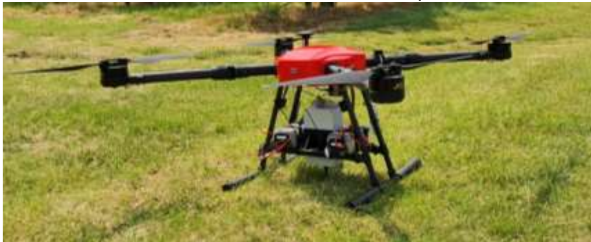
Figure 3: Hyperspectral Imaging System equipped on the drone
